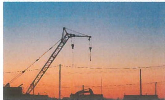
The boom on this crane must be lowered to comply with the clearance distance.
