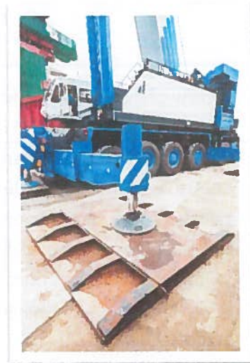
Outrigger and stabilizer blocking must be the correct size, amount, and condition.
